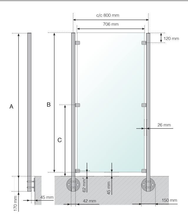
A - The total height of the wind protection from the floor surface
